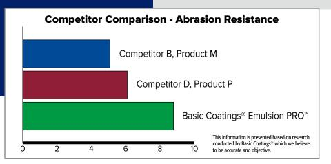
The Basic Coatings<sup>®</sup> research team conducted several abrasion tests on Emulsion PRO<sup>®</sup> against the competition. Basic Coatings could easily differentiate finish wear properties by using a combination of Taber Abraser numbers, Gardner brush cycle tests, falling sand tests and external side-by-side gloss loss tests. The results were compiled and presented on a scale of 1 to 10, with 10 being the most resistant to abrasion and 1 being the least resistant.
